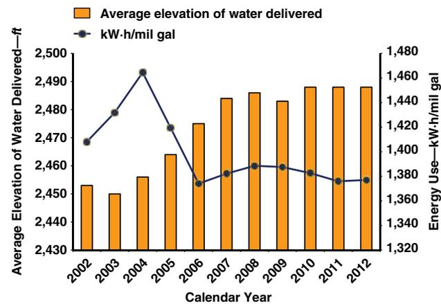
Figure shows calendar years from 2002 through 2012. Pumping plan was implemented in July 2005. Elevation of water delivered is plotted against kilowatt-hours of energy consumed per million gallons of water delivered.
